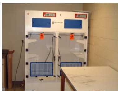
Evidence drying chamber
